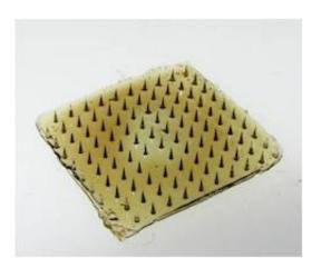
The Karp lab invented a bio-inspired flexible microneedle adhesive patch (2 x 2 cm) that can stick to soft tissues. Credit: Karp lab.
