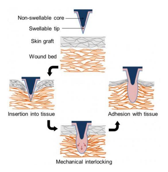
The above is an illustration of mechanical interlocking from a water-responsive dual-layered microneedle-based adhesive. Credit: Karp lab.
