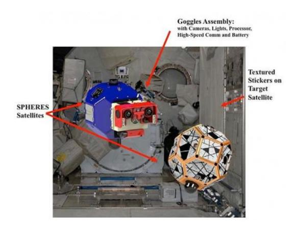
The SPHERES-VERTIGO investigation setup showing tracking (with goggles) and target SPHERES. Each satellite is an 18-sided polyhedron that is 0.2 meter in diameter and weighs 3.5 kilograms. Credit: MIT Development Team
