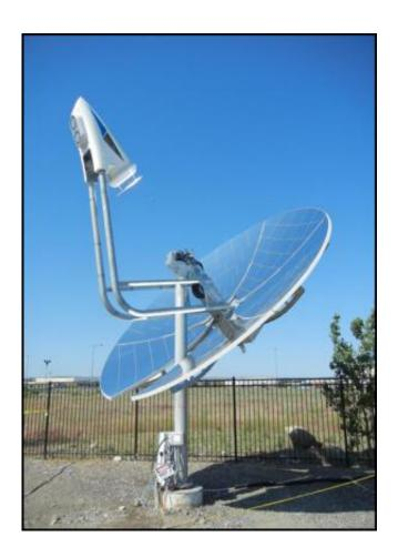
PNNL's concentrating solar power system for natural gas power plants, installed on a mirrored parabolic dish. Credit: Pacific Northwest National Laboratory
