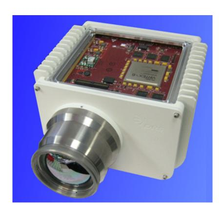
The military uses long-wave infrared (LWIR) cameras as thermal imagers to detect humans at night. These cameras are usually mounted on vehicles as they are too large to be carried by a single warfighter and are too expensive for individual deployment. However, DARPA researchers recently demonstrated a new five-micron pixel LWIR
