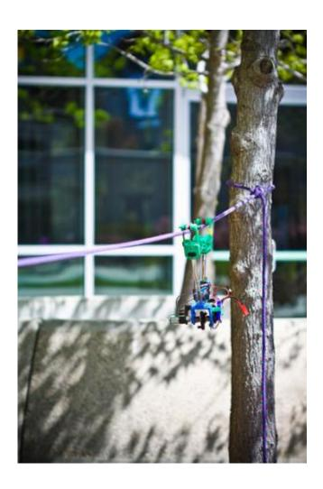
SkySweeper is V-shaped with a motor-driven "elbow" and its ends are equipped with clamps that open and close as necessary to move it down utility lines, searching for damage, inch by inch. It was designed by graduate student Nick Morozovsky in the Coordinated Robotics Lab led by mechanical and aerospace engineering professor Tom Bewley. Credit: UC San Diego Jacobs School of Engineering.
