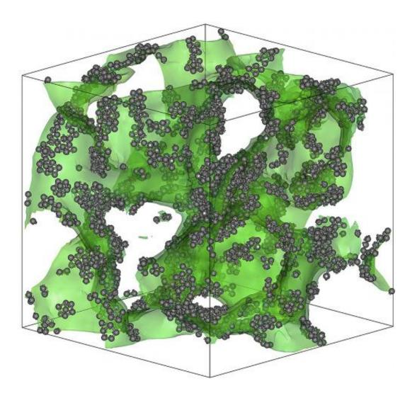
In a 50/50 mix of copper and niobium, regions that are richer in copper separate from regions that are richer in niobium. The interface between these two kinds of regions forms an irregular sponge-like surface, shown in this visualization in green. While most of the material is disordered (making it a glass), small collections of atoms at the boundary zone (shown in gray) form a stiff
