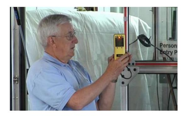
Harvey Manbeck, distinguished professor emeritus of agricultural engineering, demonstrates the use of a hand-held monitor that can detect deadly hydrogen sulfide gas in manure-storage facilities. Credit: Penn State
