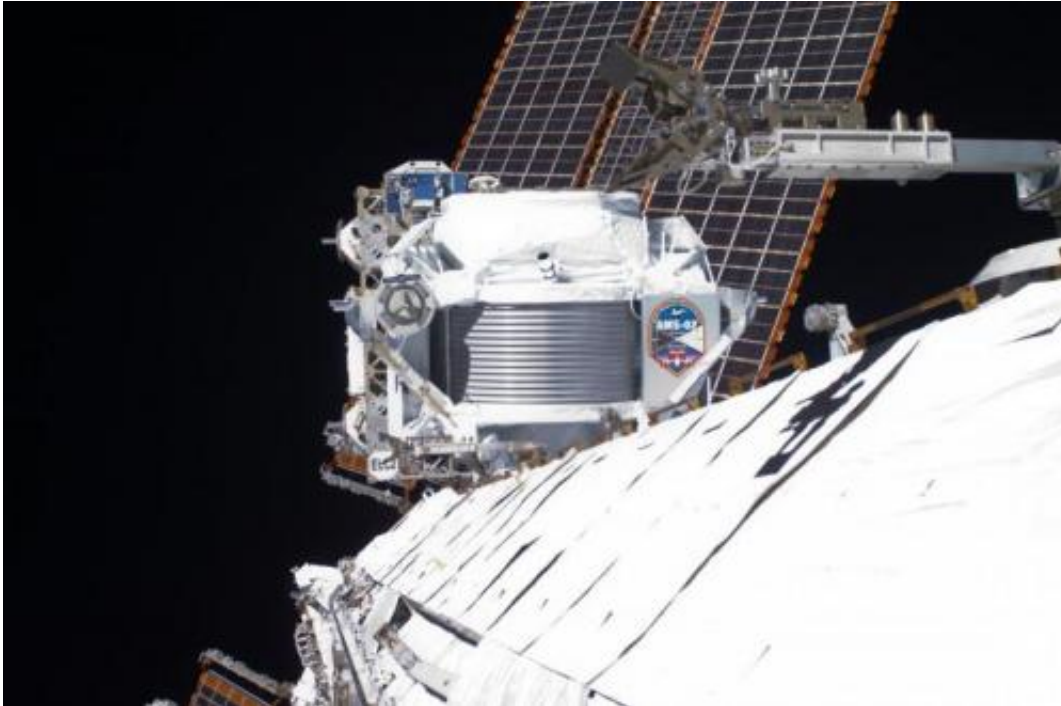
Figure 1: From its vantage point ~260 miles (~400 km) above the Earth, the Alpha Magnetic Spectrometer (AMS) collects data from primordial cosmic rays that traverse the detector.
