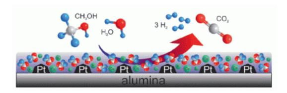
(Phys.org) —The storage of hydrogen in the form of methanol is a highly promising method for using excess energy produced by wind and solar power plants. However, this technology requires an effective catalyst for regenerating the hydrogen. German scientists have now introduced a new platinum catalyst for this reaction, known as the steam reforming of methanol, in the journal *Angewandte Chemie*. The secret of their success lies in a special coating made from molten basic alkali metal salts.
