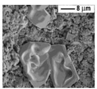
'We did index tests on the samples to find out their saturated <u>moisture</u> <u>content</u> and density and then we put them under the <u>scanning electron</u> <u>microscope</u> to look at their chalk matrix,' he explains. 'On the images we saw some really large cubic salt crystals forming in the coastal samples.'
