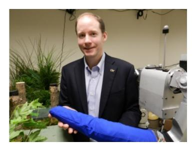
Charlie Kemp, associate professor in the Coulter Department of Biomedical Engineering at Georgia Tech and Emory University, has developed technology that keeps the robot's arm flexible and gives the robot a sense of touch across its entire arm.
