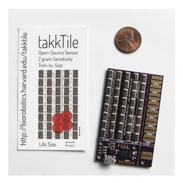
Researchers at the Harvard School of Engineering and Applied Sciences have developed a very inexpensive tactile sensor for robotic hands that is sensitive enough to turn a brute machine into a dextrous manipulator. Credit: Yaroslav Tenzer
