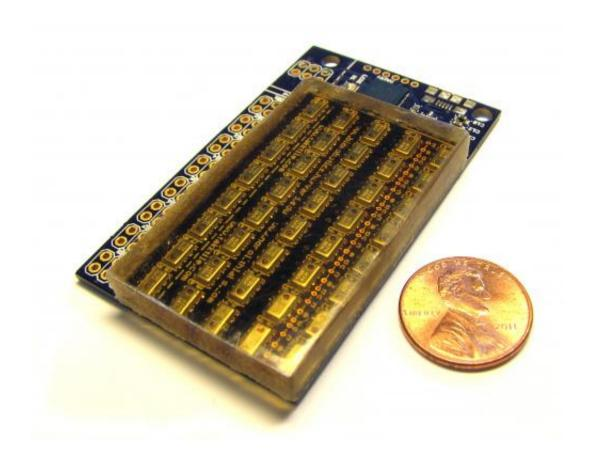
An 8x5 tactile array provides gram-level sensitivity in hardware created from MEMS barometers and standard manufacturing processes. Credit: Leif Jentoft
