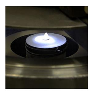
An interior glimpse of centrifugal atomization apparatus constructed at the Ames Laboratory, showing the spinning disc. The disc will intercept a stream of molten calcium and fling off a spray of fine droplets. The droplets, less than one hundred microns in diameter, solidify as they cool and are captured in a quenching bath of hydrocarbon oil, which prevents the calcium from reacting.
