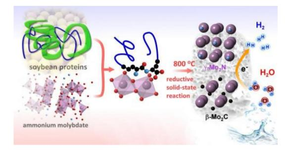
Splitting hydrogen from water: This illustration depicts the synthesis of a new hydrogen-production catalyst from soybean proteins and ammonium molybdate. Mixing and heating the ingredients leads to a solid-state reaction and the formation of nanostructured molybdenum carbide and molybdenum nitride crystals. The hybrid material effectively catalyzes the conversion of liquid water to hydrogen gas while remaining stable in an acidic environment.
