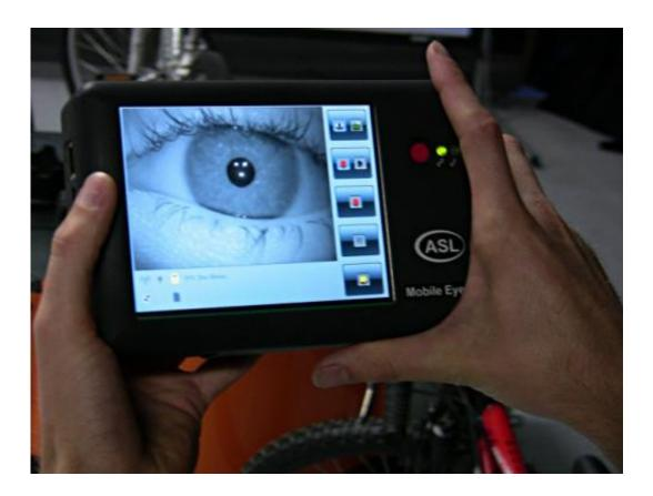
Technology can track the eye movements of a driver in a traffic simulator to determine what the person is looking at. Credit: Oregon State University
