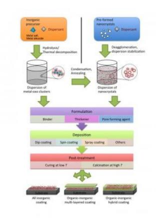
Schematic illustration in the main processing steps involved in the formation of transparent coatings containing oxide nanoparticles. Sci. Technol. Adv. Mater. Vol. 14 (2013) p. 023001. Credit: 2013 (c) L. Bergström
