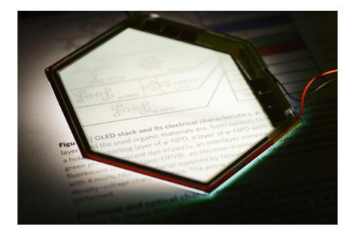
A transparent OLED made at Philips Research Aachen, seen from the rear; light is emitted from the front. Researchers at TU/e and other institutes have developed a tool that allows the light color of OLEDs to be predicted precisely. Credit: Bart van Overbeeke
