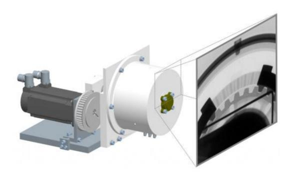
At PSI, the metal casing of a motorcycle clutch was illuminated with neutrons, in order to make the distribution of oil visible. In contrast to X-rays, neutrons pass through the metal virtually unimpeded, and will only be absorbed by the lubricating oil.
