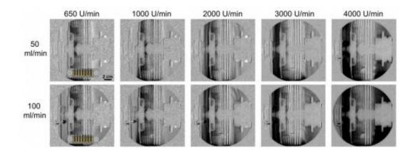
Neutron radiography shows that only the first three clutch discs are supplied with sufficient amounts of oil, regardless of the speed or oil flow rate (the lamellae are numbered from left to right).
