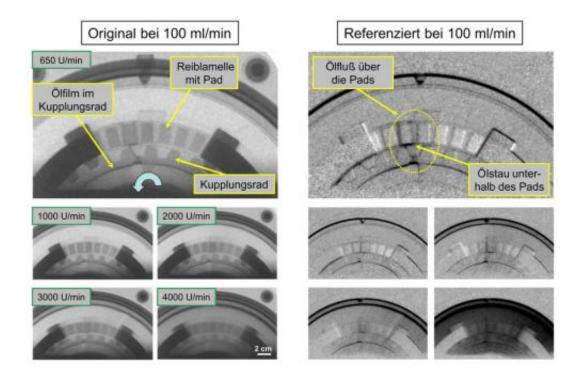
The front view shows that oil accumulates below the friction pads, and then flows out along both sides of the lamella. On the right, references were made by recording two images, the first without and then with oil. The images show only
