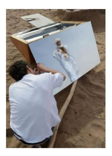
A scientist shows a nomad how to assemble a waterpod near the village of M'Hamid El Ghizlane in Zagora on March 16, 2013. There are high hopes for the waterpod, one of which can produce six litres of pure water daily from 12 litres of brackish water, according to its creators.
