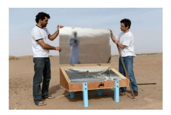
Scientists show a nomad (in reflection) how to assemble a "waterpod" near the village of M'Hamid El Ghizlane in Zagora on March 16, 2013. The "waterpod" allows desert-dwellers to turn water extracted from wells into clean drinking water through evaporation and condensation.
