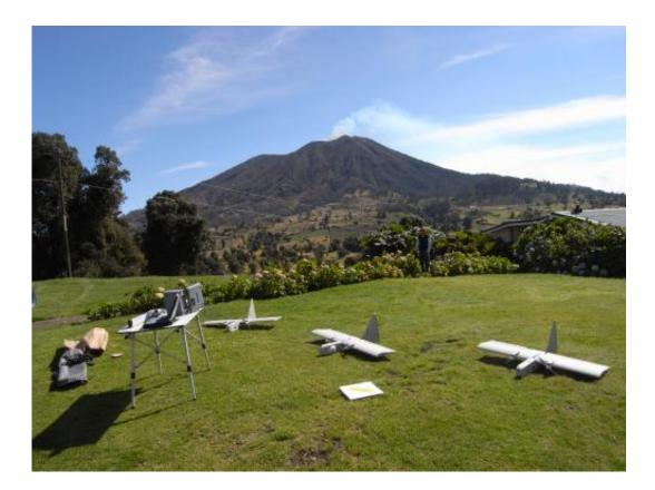
NASA researchers modified three repurposed Aerovironment RQ-14 Dragon Eye unmanned aerial vehicles acquired from the United States Marine Corps to study the sulfur dioxide plume of Costa Rica's Turrialba volcano. The project is designed to improve the remote sensing capability of satellites and computer models of volcanic activity. Credit: Google/NASA/Matthew Fladeland
