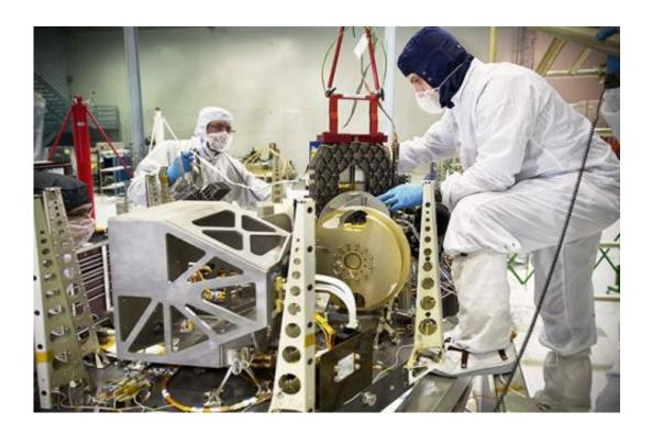
Engineers prepare and install the Microshutter Array simulator onto the NIRSpec Engineering Test Unit at NASA Goddard Space Flight Center. Credit: NASA/Chris Gunn
