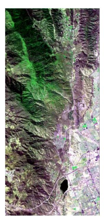
The HyspIRI airborne campaign overflew California's San Andreas Fault on March 29, 2013. The three-color (red, green, blue) composite image of the fault, composed from AVIRIS data, is similar to what a snapshot from a consumer camera would show. The entirety of data from AVIRIS, however, spans the visible to the short-wavelength infrared part of the spectrum. Credit: NASA
