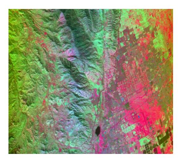
Temperature information was collected simultaneously by the MASTER instrument. Red areas are composed of minerals with high silica, such as urban areas, while darker and cooler areas are composed of water and heavy vegetation. Credit: NASA
