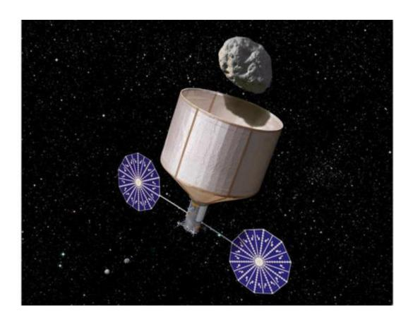
This mission is a concept under study by NASA that would - for the first time - capture and relocate a ~500,000-kg Near Earth Asteroid (NEA) to high lunar orbit. The capture, transportation, examination, and dissection of an entire NEA would provide valuable information for planetary defense and a unique, meaningful, and affordable destination for future robotic and human exploration. Credit: Rick Sternbach / KISS
