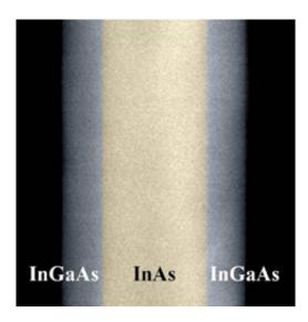
A false-color microscope image of a single nanowire, showing the InAs core and InGaAs shell. Credit: Parsian Mohseni
