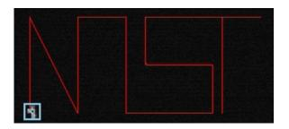
Video showing a 10  $\mu$ m × 1  $\mu$ m fluorescently labeled rod being controlled using a combination of electric fields and fluid flow to travel along the "NIST" path, graphically underlaid in red. The rod is made to simultaneously rotate and align itself tangential to each of the 12 line segments by the time its center of mass reaches the end of a segment. The imaged area is 160  $\mu$ m × 70  $\mu$ m.
