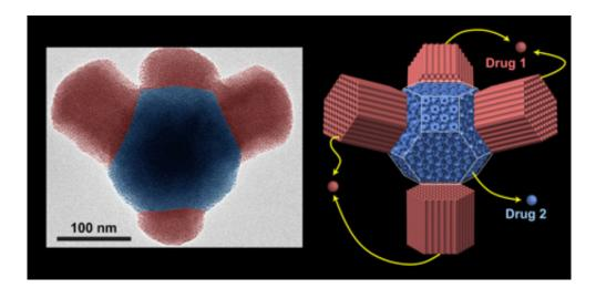
This false-color image (left) depicts the core lattice in blue, where drugs can be placed in compartment pores for targeting in the body. In the hexagon-shaped cylinder branches, other types of drugs may be place for delivery. Simultaneous delivery of pharmaceuticals can thus be optimized for each drug separately. The accompanying illustration (right) offers a clear vision of the left image. Credit: Wiesner Lab
