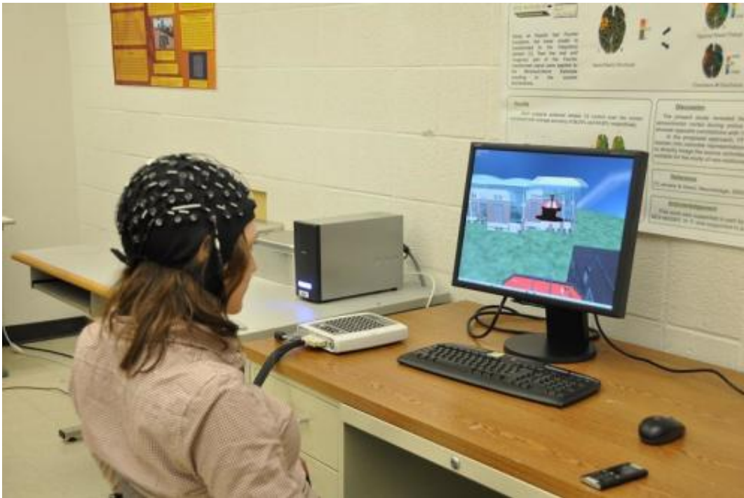
User controls flight of a 3-D virtual helicopter using brain waves. Credit: Bin He, University of Minnesota
