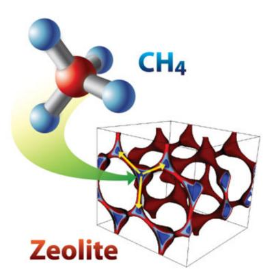
This image shows methane capture in zeolite SBN where blue represents optimal adsorption sites for methane uptake and yellow arrow shows interaction distance. Credit: Berend Smit
