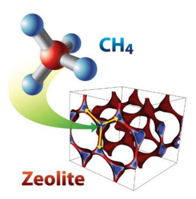
Methane capture in zeolite SBN. Blue represents adsorption sites, which are optimal for methane (CH4) uptake. Each site is connected to three other sites (yellow arrow) at optimal interaction distance.
