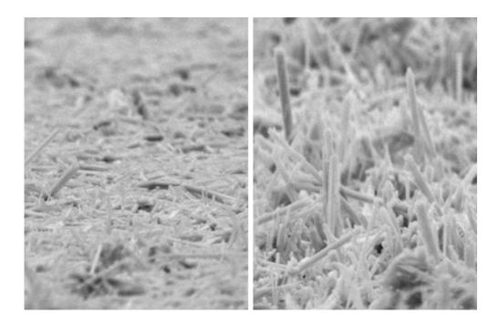
The non-aligned manganese dioxide nanorods on the left were made using conventional methods. The aligned nanorods on the right were grown in Desheng (Dennis) Meng's lab at Michigan Technological University using electrophoretic deposition. Using aligned nanorods, Meng's group was able to build a superior chemical capacitor. Credit: Sunand Santhanagopalan
