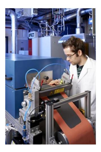
Roll-to-roll coating of electrodes at IWS: The scientists now have optimized the design of anode and cathode for lithium-sulfur batteries. Credit: Jürgen Leibmann
