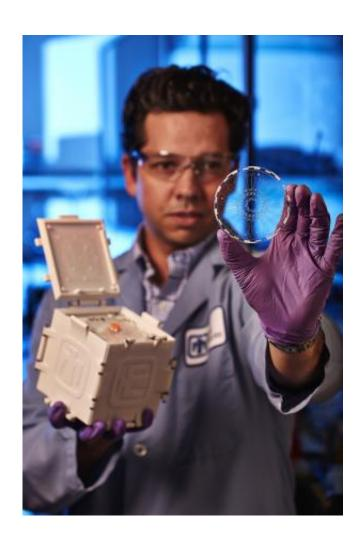
Sandia's SpinDx device features centrifugal microfluidics, or "lab-on-a-disk" technology, which uses centrifugal forces to manipulate samples and reagents through microfluidic channels implanted on disks that are of the same size as a standard CD or DVD. Credit: Jeff McMillan
