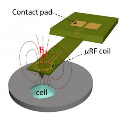
This image illustrates the concept for a new type of technology that combines two biological imaging methods -- atomic force microscopy and nuclear magnetic resonance -- to create a new way to study cancer-cell metastasis and other disease-related processes. (Purdue University image/ Xin Xu) Credit: Purdue University/ Xin Xu
