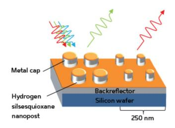
Variation in post size and spacing in the metal array alters which incoming wavelength of light (red, green or blue) is reflected back. Reproduced from Ref. 1 © 2012 K. Kumar et al.
