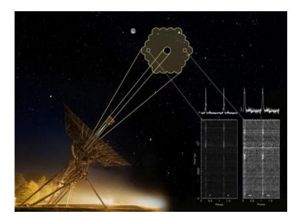
The new field of view (the large hexagon) of the Apertif receivers on the Westerbork telescope is thirty times bigger than the old one (central circle) and the full moon. With the new high-speed cameras, astronomers will be able to detect weak and rare cosmic flashes. Recently, with the test system, two fast blinking pulsars have already been observed simultaneously. These flashes are visible at the bottom right.
