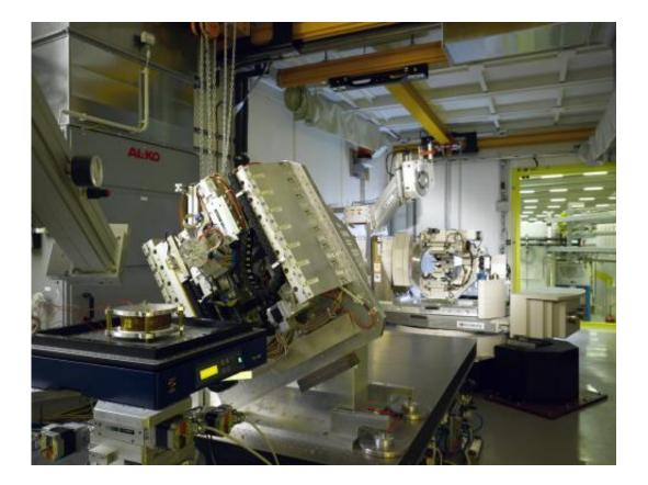
The LISA diffracometer at DESY: the instrument deflects the brilliant X-rays of DESY, thus allowing scientists to investigate interfaces of liquid samples (on the left). Credit: DESY
