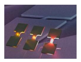
Light emitting bridges of germanium can be used for communication between microprocessors. Credit: Hans Sigg, PSI
