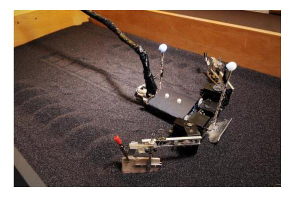
FlipperBot moves through a bed filled with poppy seeds in the Georgia Tech School of Physics. The research, which also included a study of sea turtle hatchlings, provides new information on the principles governing locomotion on granular surfaces. Credit: Gary Meek
