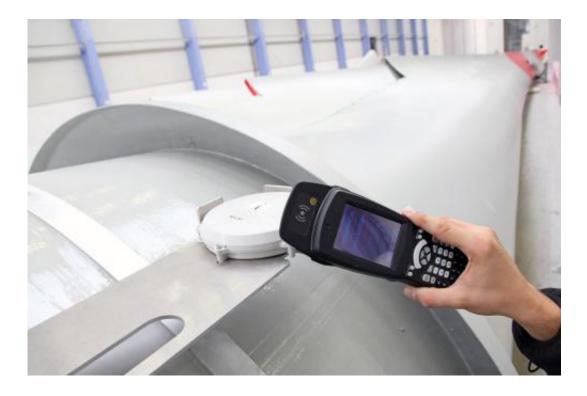
RFID chips in the module and in the locator make automatic continuous tracking possible. Credit: Dirk Mahler
