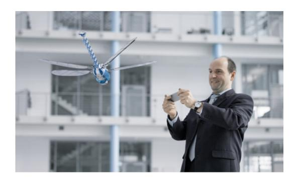
(Phys.org) —German technology company Festo has unveiled the BionicOpter, a fully functional robotic dragonfly. It can fly forwards, backwards, hover and even fly sideways—just like a real dragonfly. Its introduction marks another step forward in robotics engineering.
