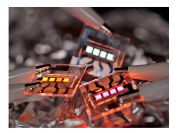
Organic light emitting devices are surface beamers that can be applied even onto flexible substrates in a very thin coating. Particularly when it comes to very bright light levels, non-homogeneities can occur with self-heating. Photo: IAPP
