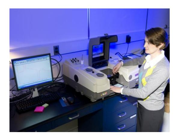
Christina Hacker characterizes the individual monolayers prior to flip-chip lamination using a Fourier transform infrared spectrometer.
