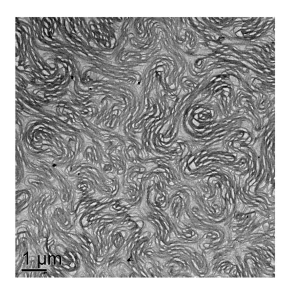
A web-like, gel structure is formed after fluid passes through the flow device. The unit of measurement is 1 micron. Credit: Environmental Molecular Sciences Laboratory and University of Washington
