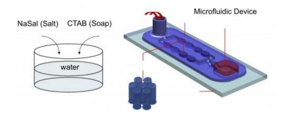
This is a diagram showing how the microfluidics device works. Water mixed with salt and soap is injected into a spout (left back). The fluid travels through a series of posts (see enlarged segment) that cause the fluid to thicken. Credit: University of Washington
