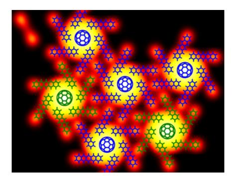
UHV STM image of C60-Pn in-plane chiral heterojunctions, overlaid with molecular models showing the orientation and the chirality (right-handed green, left-handed blue) (middle).
