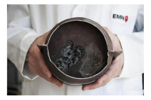
This honeycomb catalyst from a racing car was the trigger which gave the Empa researchers the idea of developing the Foamcat. A small area of the monolith has melted, but neighboring areas are almost unused, indicating that the exhaust gas flow is poorly distributed through the device. Credit: Empa
