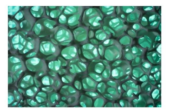
The irregular structure of the ceramic foam substrate causes the exhaust gas to flow in a turbulent manner, improving flow distribution and therefore reducing the quantity of noble metals required for catalysis. Credit: Empa
