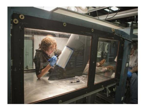
Bug team researcher John Gardner lies inside the Basic Aerodynamics Research Tunnel, or BART, to prep leading edge of a scale model wing for a blast of bugs from the tunnel's bug "gun." Credit: NASA
