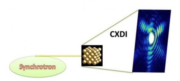
Highly coherent X-rays from synchrotron sources can be used for imaging nanomaterials in 3-D at tens of nanometer of spatial resolution. This image shows a monochromatic hard X-rays patterns from a single crystal gold particle, which produces a speckle-like fringe image. Inverting such "diffraction images" under certain conditions can result in a high-resolution distribution of the electron density (amplitude) and strain of the lattice structure (phase shift). Credit: Wenge Yang
