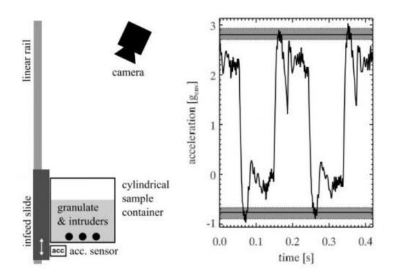
Left: Sketch of the experimental setup. The sample container is attached to an infeed slide, which can be moved vertically on a linear rail. Right: Acceleration profile of the infeed slide and the attached experiment container for an experiment with  $g_{amb} = g_{Mars}$ . Credit: arXiv:1304.0569 [cond-mat.soft]
