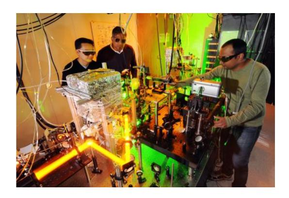
A team of Georgia Tech researchers adjusts equipment used to study a gaseous Bose-Einstein condensate composed of sodium atoms. The condensate could be used for communicating among quantum computers. Shown, (l-r) are postdoctoral fellow Carlo Samson, associate professor Chandra Raman and graduate student Anshuman Vinit. Credit: Gary Meek
