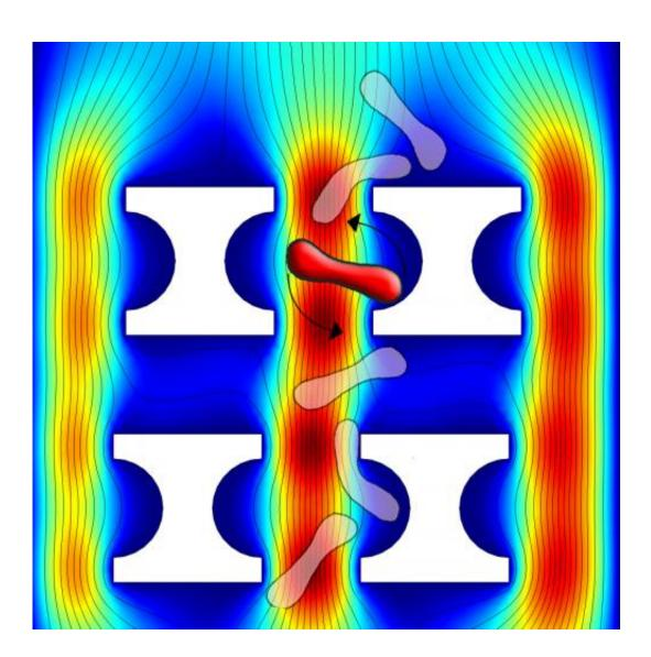
How the I-shape pillar array works. Non-spherical cells such as rod-shaped ones are rotated by I-shape pillar to increase their effective hydrodynamic size,
